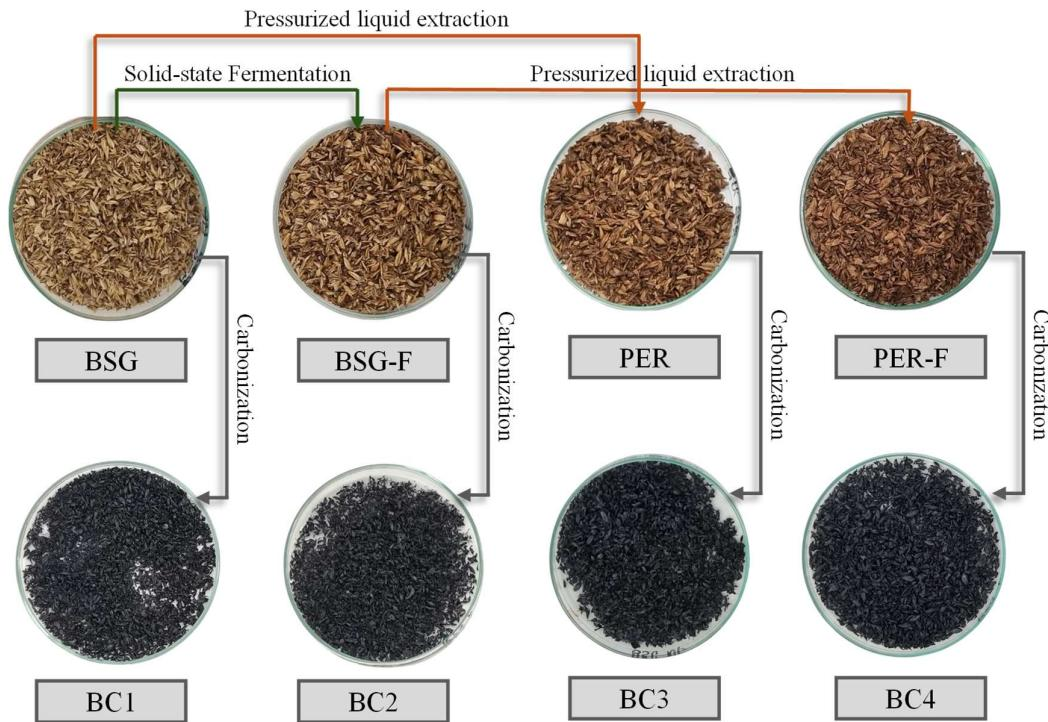
Figure 1. Samples that were tested as adsorbents and the processes they underwent.
