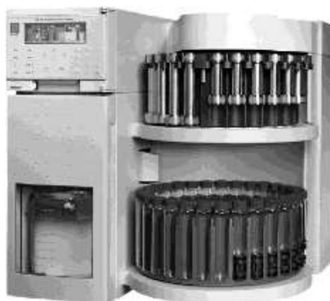
Figure 1.5. Pressurized liquid apparatus used in Grisales-Mejía et al., (2024)
