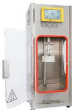
Figure 1.2. Probe ultrasound apparatus used in Bezerra et al., (2024)
