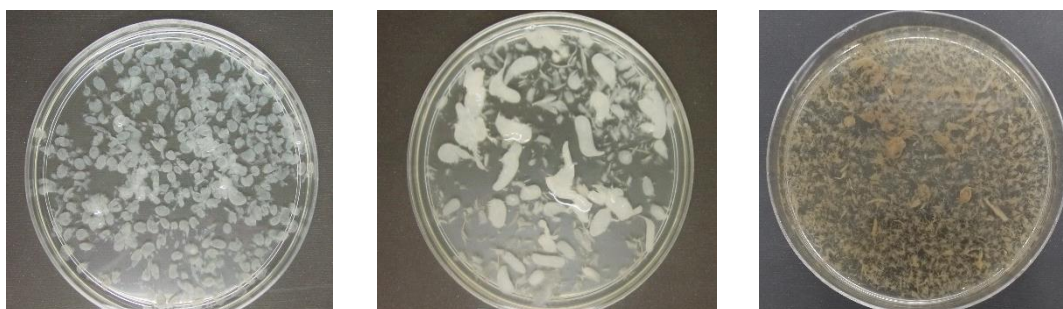
Figure 2: BC formed using stirrer a) HS medium with ethanol b) HS medium without ethanol c) CSM medium without ethanol
